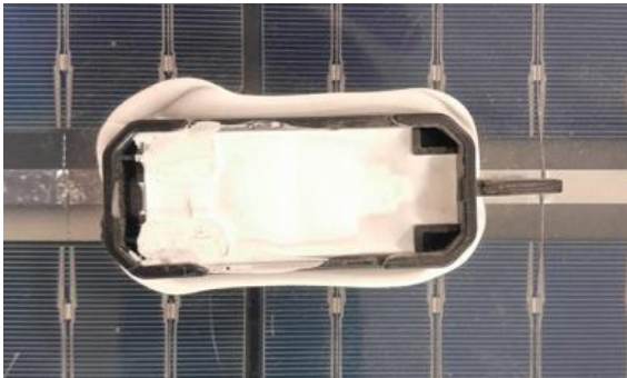
Junction Box opened view
